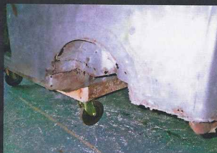
After blasting: "Once blasted, make sure you prime the whole vehicle as it started to rust and we had to have it blasted again."
