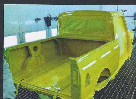
"The Inca Yellow was chosen because, when we sandblasted it back through the layers (which looked like a stick of rock) the very last colour was yellow."
