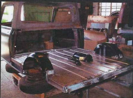
New rear floor and arches in place before rear bulkhead was welded in. Precise panel alignment is the big challenge here.
