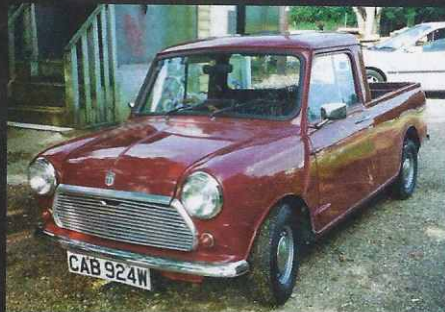
"Shell was sandblasted by ourselves, which was a real bonus, but did it unearth some bloody big holes. Most of the old repairs had been stuck on and filled over."
